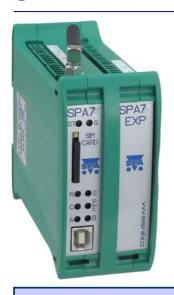
Both SPA7 and SPA7-GPRS are expandable by a SPA7-EXP board, which increases the number of inputs/outputs by 10 analog inputs, 4 logical outputs and 2 analog outputs and RS232/485 serial port. This expansion must be done only by a manufacturer, due to necessity of recalibration of the connected modules. Does not order separately; must be ordered together with SPA7!
